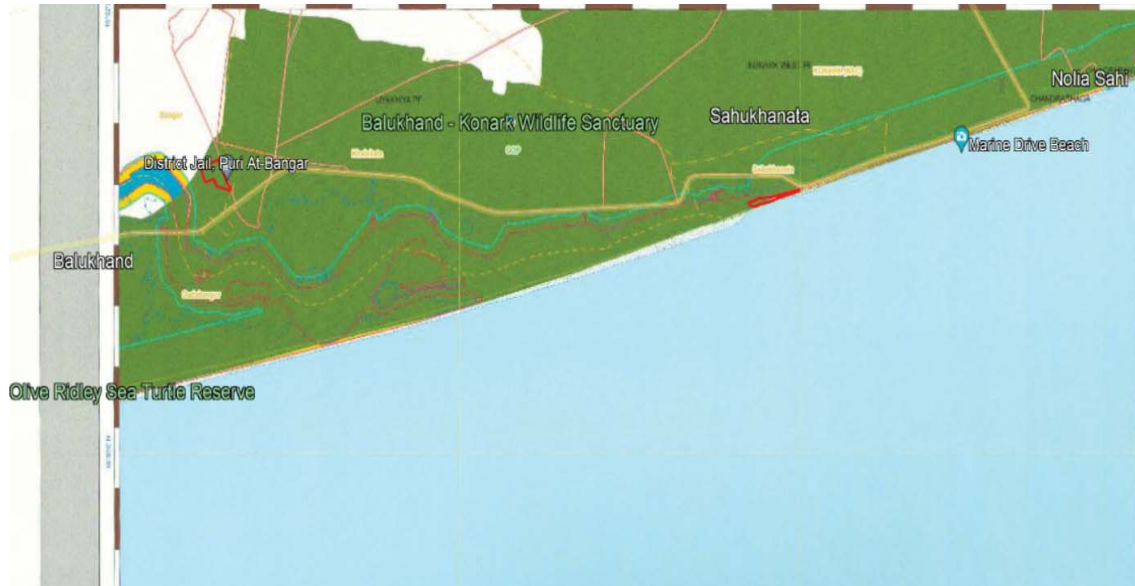
Fig. 4: CZMP for the coast around Balukhand sanctuary and Turtle reserve, indicating CRZ 1A zone in green shade and irregular construction is marked in red
